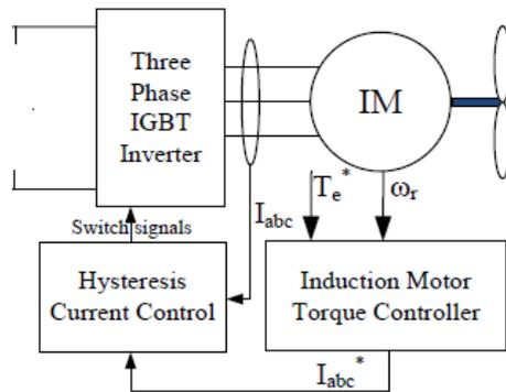
**Figure 4:** Propulsion motor and drive block diagram
