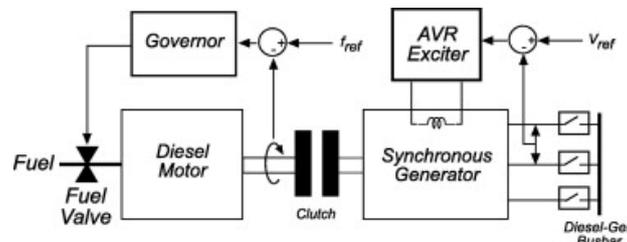
**Figure 2:** Diesel Generator Set block diagram
