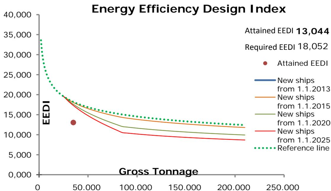
Figure 5: EEDI of the ship under study in contrast to reference lines of IMO.
