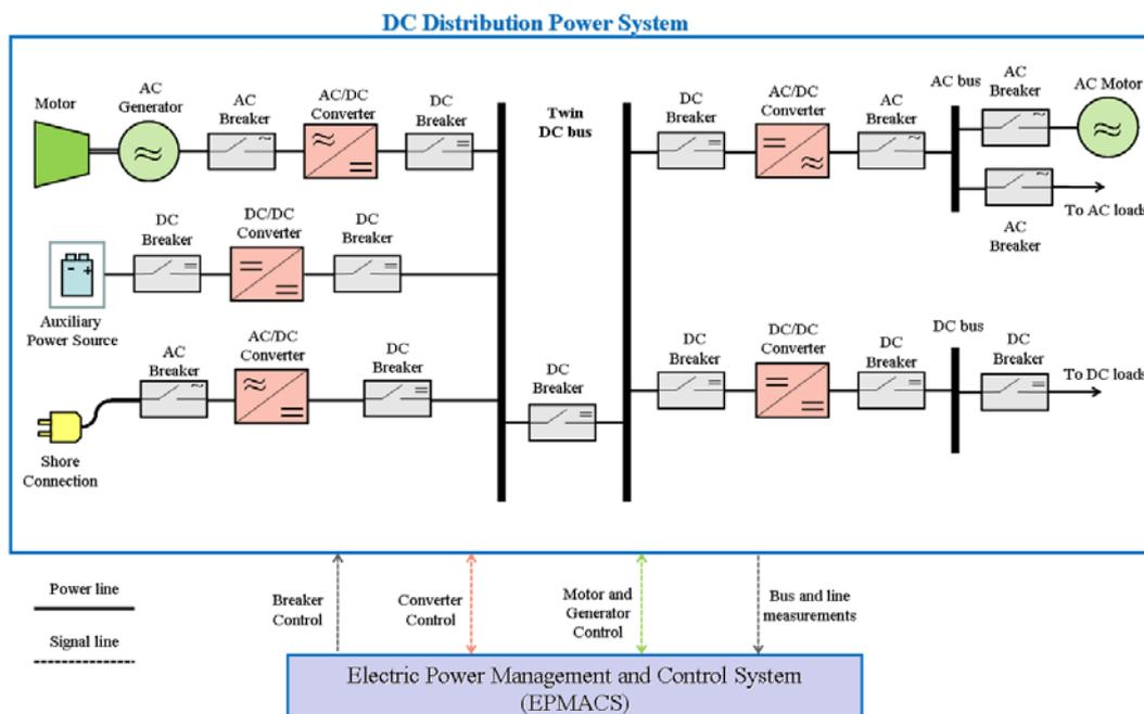
**Figure 1:** Conceptual DC Distribution Power System
