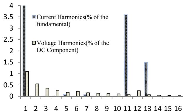
Figure 5 : Fourier Analysis of AC Current and MVDC Voltage
