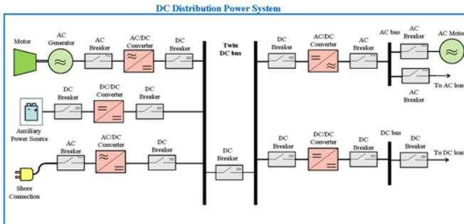
Figure 1: Conceptual DC Distribution Power System
