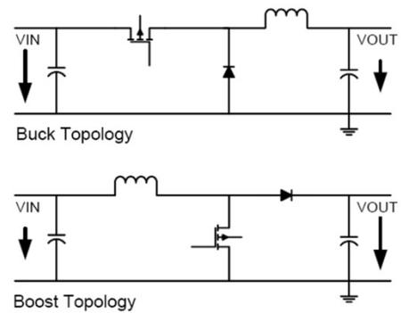
Figure 4 : Buck and Boost Converter Topologies
