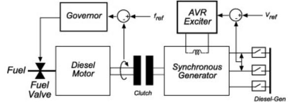
Figure 2: Diesel Generator Set block diagram
